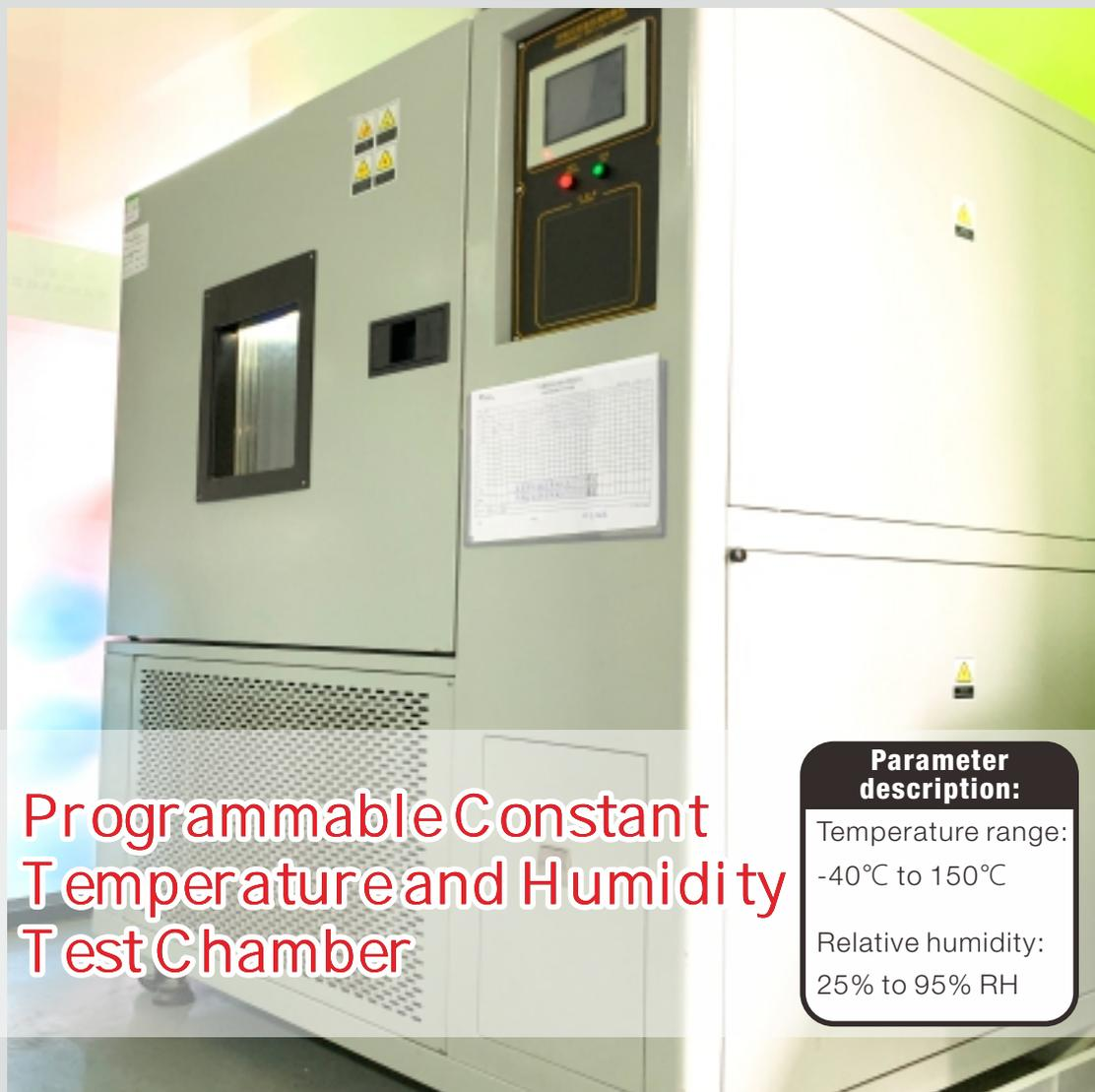
Programmable constant temperature and humidity test chamber is necessary test equipment in the fields of electrical appliances, aviation, automobiles, household appliances, coatings, chemicals, scientific research and so on. It is used to test and determine the parameters and performance of electrical, electronic and other products and materials and surface treatment after temperature environment changes in high temperature, low temperature, humidity and heat degree or constant test.
